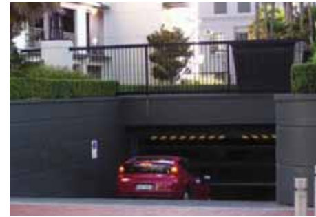
Basement carparking maximises the development potential of ground floor space and allows for a continuous built edge at the street level.
