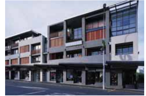
The façade of this development is broken up to reduce its perceived size and bulk. The use of a variety of materials provides interest and articulation whilst the 'floating' roof adds lightness.
