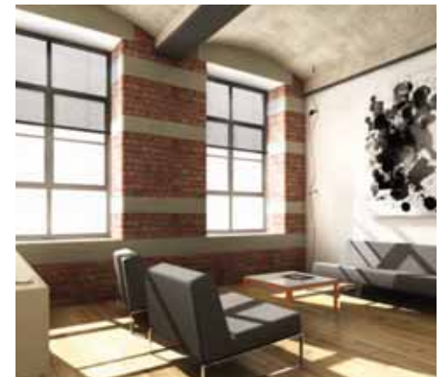
Incorporating a large amount of floor area within 4–6m of an external window ensures maximum sunlight penetration into a development. [Image courtesy of Urban Splash, UK.]
